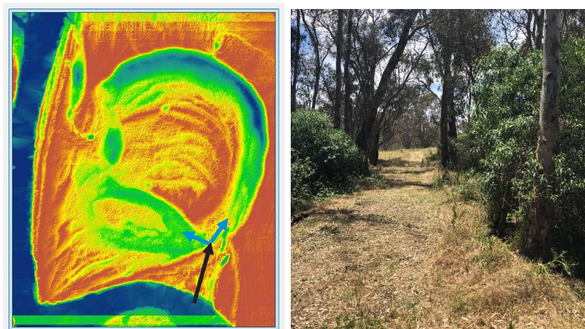
Figure 12: Left hand picture shows a DEM of Horseshoe Lagoon; black arrow shows the proposed location of a temporary pump, blue arrows show the direction of water delivery. Right hand picture shows the site conditions proposed pumping point (December 2018).
